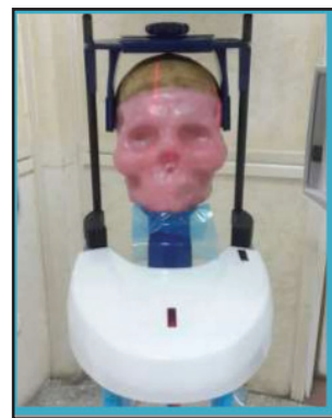
Figure(1) Photograph showing a dry human skull with soft tissue simulation using pink wax mounted on CBCT Planmeca ProMax 3D Mid machine.
