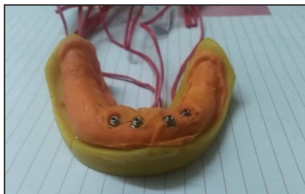
Figure (4): Strain gauge installed
