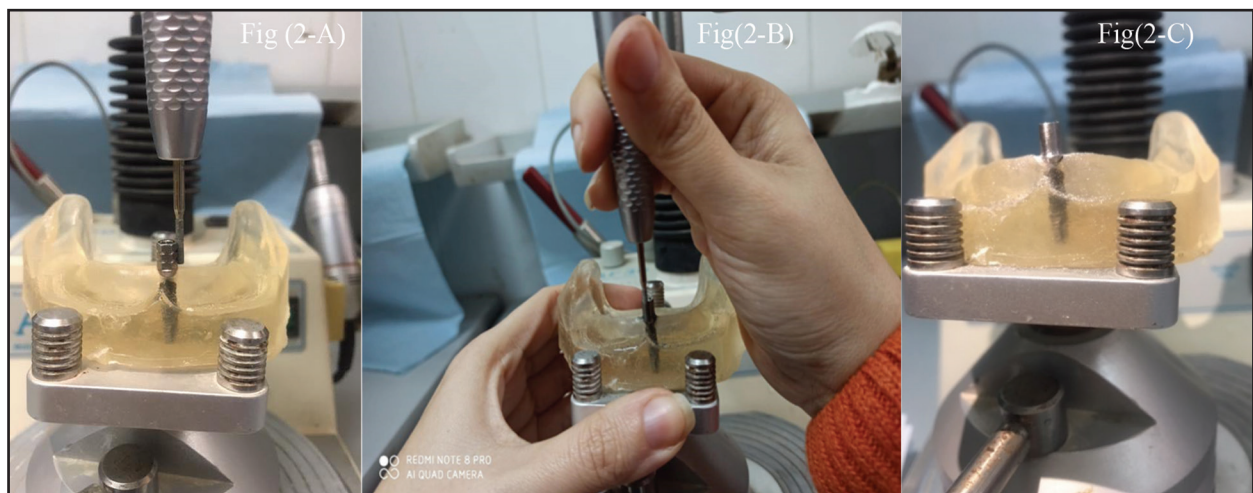
Figure (2) A) The cast is attached to the table of milling machine , B) Reduction is carried out with minimum thickness 6mm reduction is carried out, C) Finished abutment reduction
